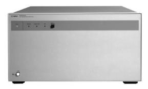
The Agilent E5250A Low Leakage Switch supports non-Kelvin measurement on four SMUs, with six additional multiplexed inputs for other needs. Besides supporting traditional matrix functionality (Agilent E5252A cards), the E5250A also supports long-term reliability stress testing (Agilent E5255A cards). The E5250A can be configured with one to four output cards or either type. The E5250A also supports a VXI*plug&play* driver for easy programmatic control.
