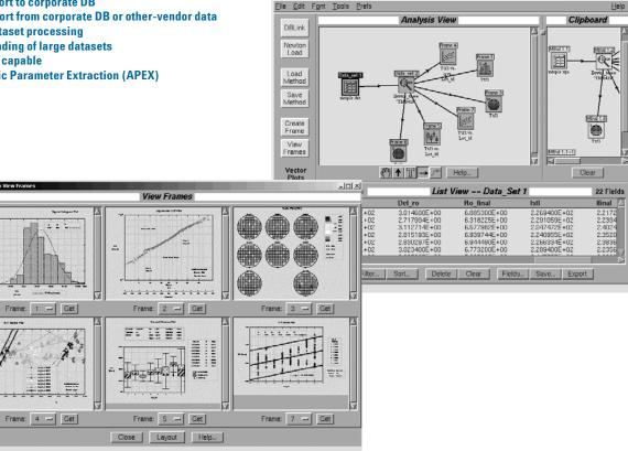
Agilent ASUR RDA is post-test statistical and physical analysis software. It aids in the analysis of production, development or qualification test data taken by the Agilent ASUR test software.
